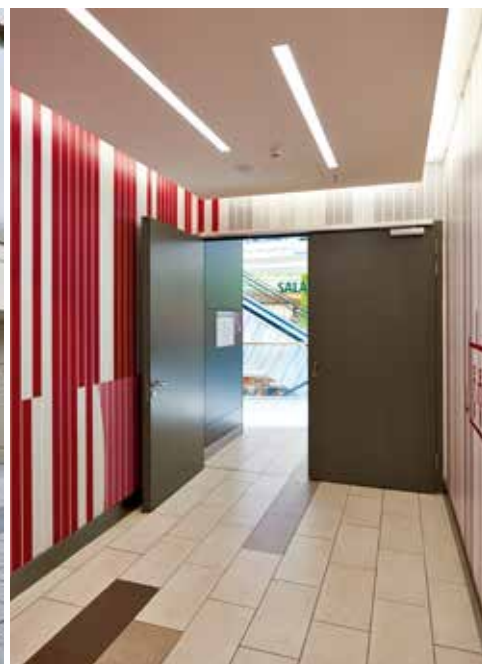
External door with ventilation slats. Double-leaf fire-rated and smoke-tight doors protect the escape routes to the outside.
